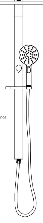
Note: This shower has a WELs certified flow restrictor fitted to the handpiece (see diagram 5). If you want a greater flow, remove this disc but note that this will not give a WELS 3-star water rating anymore.
