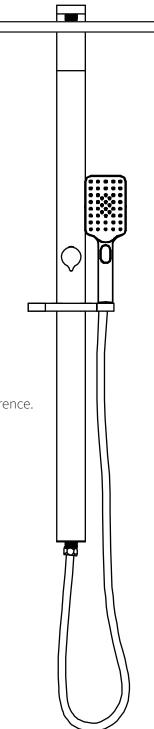
Note: This shower has a WELs certified flow restrictor fitted to the handpiece (see diagram 5). If you want a greater flow, remove this disc but note that this will not give a WELS 3-star water rating anymore.
