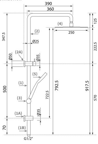
\*FOR PRESSURES EXCEEDING 500kPa INSTALL A PRESSURE REDUCING VALVE. THOROUGHLY FLUSH ALL PIPES TO **ELIMINATE ANY REMAINING DIRT AND RESIDUE, AND INSTALL** INLINE FILTERS. FAILURE TO DO SO MAY VOID THE WARRANTY.
