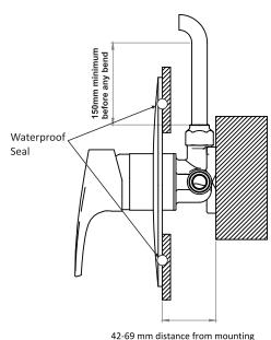
42-69 mm distance from mounting stud to outside face of wall lining
